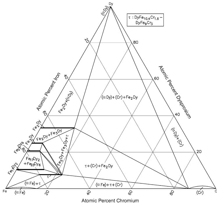
**Fig. 1** Cr-Dy-Fe isothermal section at 500 °C [2009Yao]. Narrow two-phase regions are omitted
